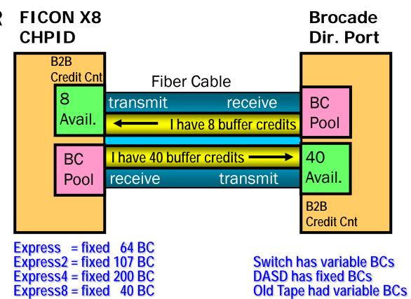
Each receiver on the fiber cable can state a different value!
