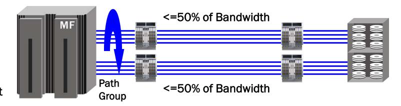
But each fabric really needs to run at no more than 45% busy so that if a failover occurs then the remaining fabric can pickup and handle the full workload z/OS's IOS automatically load balances the FICON I/O across all of the paths in a Path Group (up to 8 channels in a PG)
